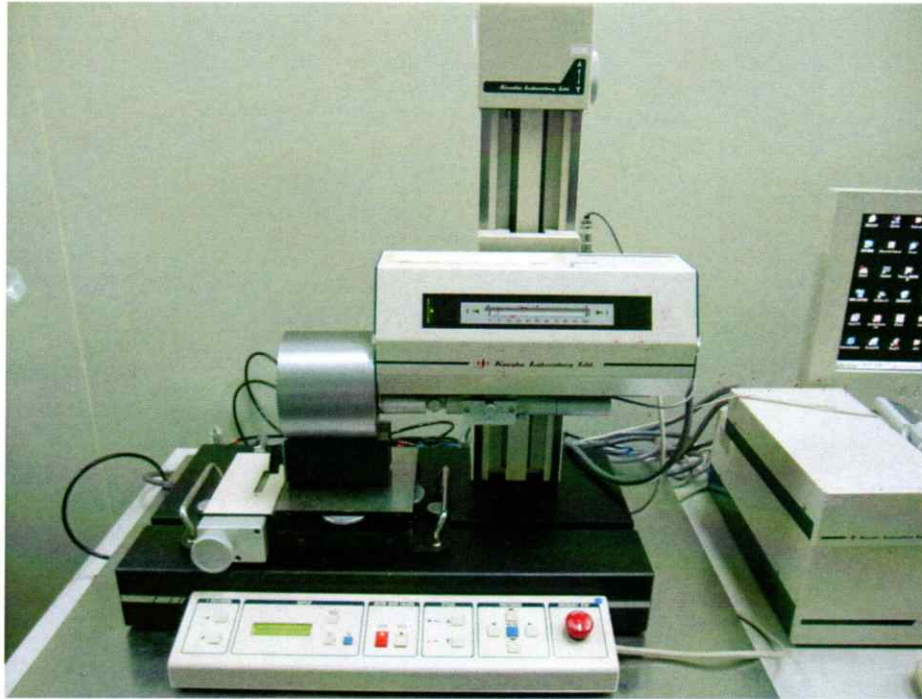
Figure 3-2-4 Actual measurement of surface roughness of the workpiece
