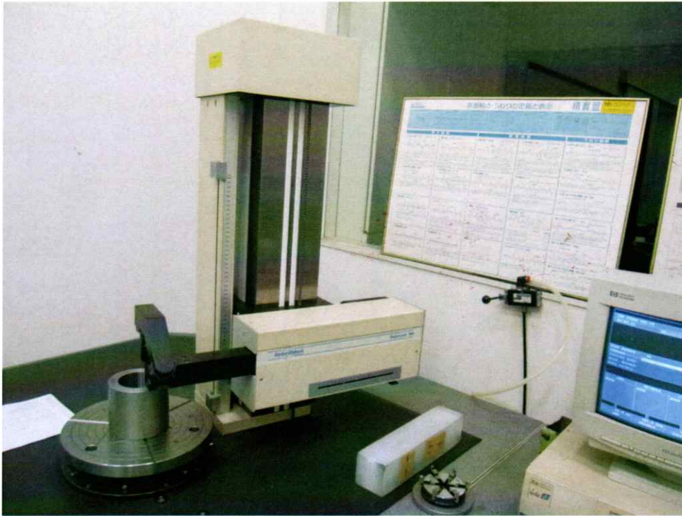
Figure 3-2-6 Actual measurement of machining roundness of the workpiece
